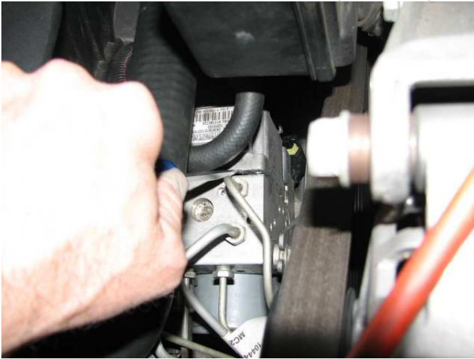
Figure 12: Separating the EBCM from the Brake module
